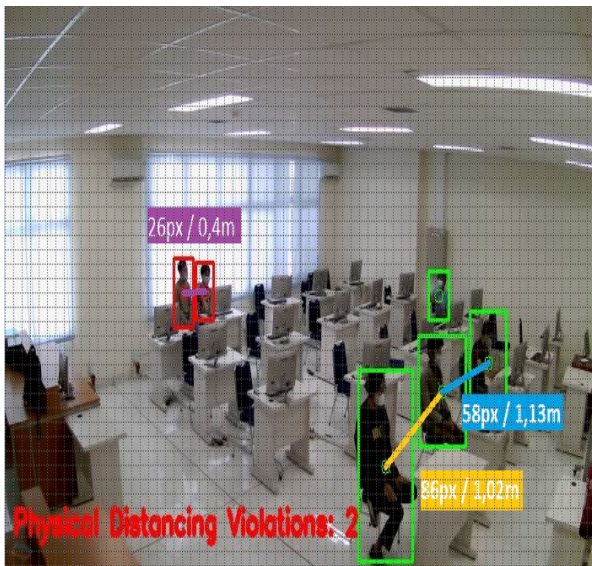
Fig. 5. Measurement of actual distance vs number of pixels
